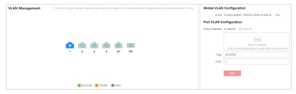
**Figure 4-11 Configure Port VLAN**
