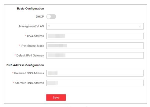
**Figure 2-2 Modify Network Parameters**
