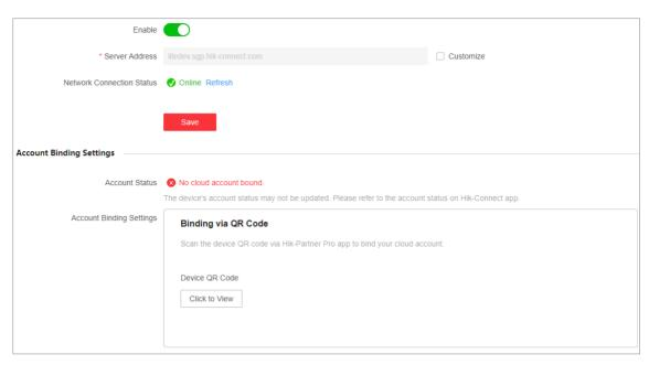
**Figure 5-9 Configure Cloud Platform**
