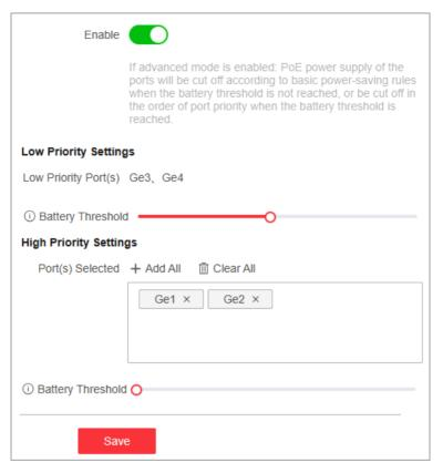
Figure 4-36 Configure Advanced Power Saving Mode
