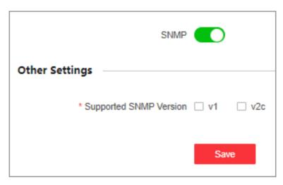
**Figure 4-16 Configure Basic SNMP Parameters**
