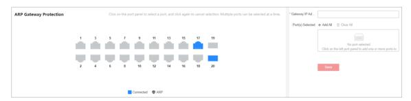
Figure 4-27 Configure ARP Gateway Protection
