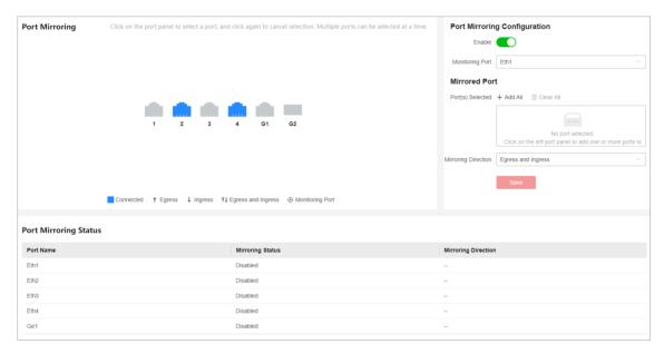
**Figure 4-4 Configure Port Mirroring**
