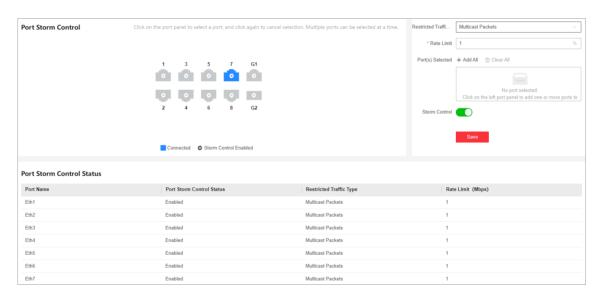
**Figure 4-7 Configure Port-Based Storm Control**
