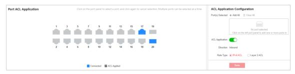
Figure 4-26 Configure Port ACL Application
