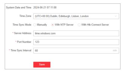
Figure 5-2 Configure Time with NTP Server
