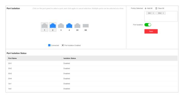
**Figure 4-3 Configure Port Isolation**
