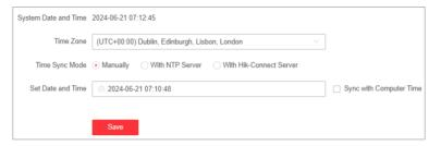
**Figure 5-1 Configure Time Manually**
